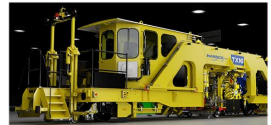
TX16 Production / Switch Tamper
